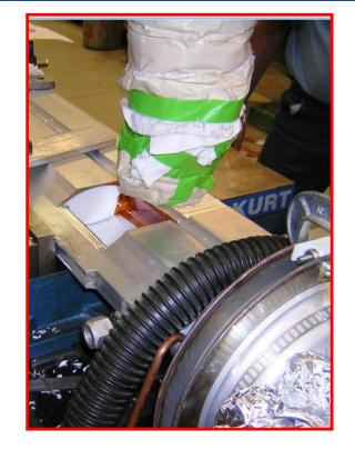
**CNC Machining Processes (with 99.5% Ethanol as lubricant)**
